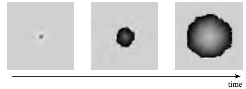
Fig. 6. Traveling nonlinear wave that is generated by the improved SE-RD device (simulated). 50 \times 50 oscillators are placed in the device. This simulation used the same parameters as in Fig. 4 (b). In this figure, high voltage is bright and low voltage is dark.
