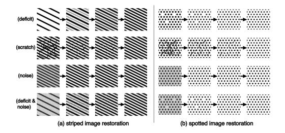
The figure above shows numerical simulation results of the proposed model demonstrating image restoration of (a) striped and (b) spotted images. The image restoring ability of the proposed model was qualitatively the same as the previous model in [3], which indicated that the image restoring based on RD computing could be performed on smart hardware; i.e., simple amplifiers and 2-D resistive sheets of polysilicon layers.
