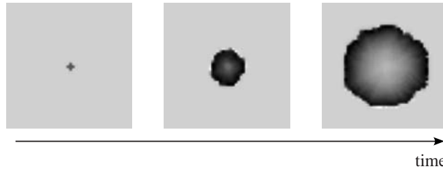
Fig. 7. Traveling nonlinear wave that is generated by the improved SE-RD device (simulated). 50 \times 50 oscillators are placed in the device. This simulation used the same parameters as in Fig. 5 (b). In this figure, high voltage is bright and low voltage is dark.
