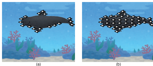
Figure 1: Motion estimation for a textureless object: (a) image of usual motion estimation, (b) image of motion estimation with spatial patterns generated
