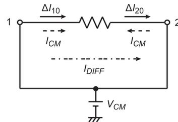
**Fig. 3** Offset currents of resistor circuit. Offset currents  $\Delta I_{10}$  and  $\Delta I_{20}$  consist of common-mode offset current  $I_{CM}$  and differential offset current  $I_{DIFF}$ .
