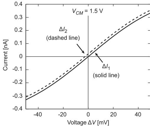
**Fig. 4** Voltage-current characteristic of resistor circuit, measured for  $I_b = 1$  nA,  $V_{dd} = 3$  V, and  $V_{CM}$  (common-mode voltage for terminals 1 and 2) = 1.5 V.
