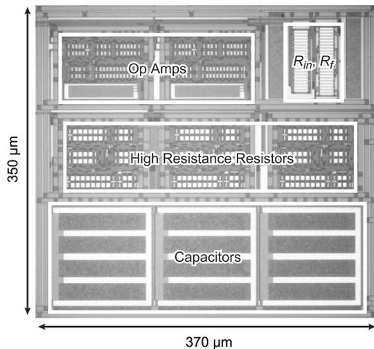
**Fig. 9** Chip photograph of phase-shift oscillator. Chip size is  $350\ \mu\text{m} \times 370\ \mu\text{m}$ . Parameters used were  $R_{in} = 5\ \text{k}\Omega$ ,  $R_f = 170\ \text{k}\Omega$ ,  $C = 10\ \text{pF}$ ,  $V_{dd} = 3\ \text{V}$ , and  $E_0 = 1.5\ \text{V}$ .
