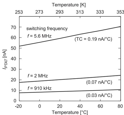
Fig. 13 Temperature characteristic of PTAT current source for three switching frequencies.
