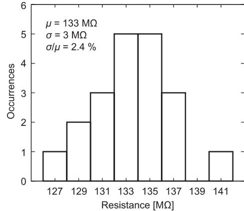
**Fig. 7** Distribution of resistance for 20 samples measured at room temperature.
