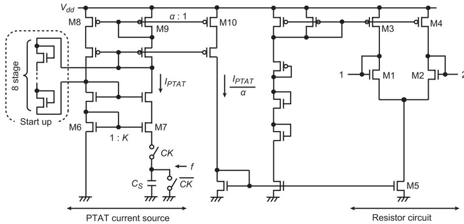
Fig. 11 Resistor circuit with temperature compensation.
