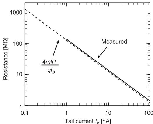
**Fig. 6** Resistance of resistor circuit as a function of bias current  $I_b$ . Solid line shows measured data, and dashed line shows theoretical resistance.
