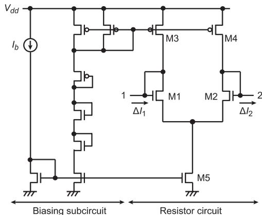
**Fig. 2** Resistor circuit with biasing subcircuit. Aspect ratio is  $20\ \mu\text{m}/4\ \mu\text{m}$  for every MOSFET.
