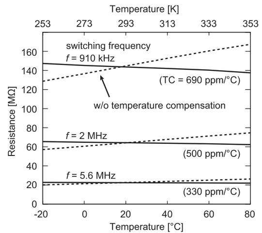
Fig. 14 Temperature characteristic of resistor circuit with compensation. Parameters used for fabrication were  $V_{dd} = 3\text{ V}$ ,  $\alpha = 10$ ,  $K = 2$ , and  $C_S = 0.55\text{ pF}$ .
