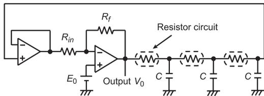
**Fig. 8** CR phase-shift oscillator. Resistors circled by dashed lines represent resistor circuits.
