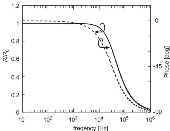
Fig. A·1 Frequency characteristic of resistor circuit.
