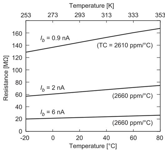
Fig. 12 Temperature dependence of resistor circuit for three bias currents.
