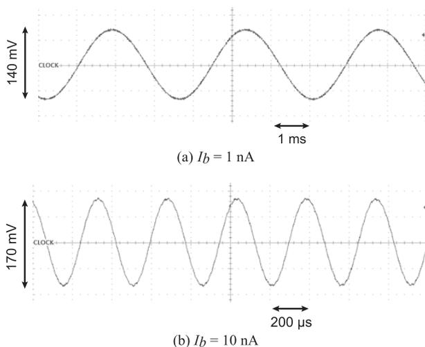
**Fig. 10** Output waveforms of phase-shift oscillator, measured for two bias current  $I_b$  values for resistor circuit.
