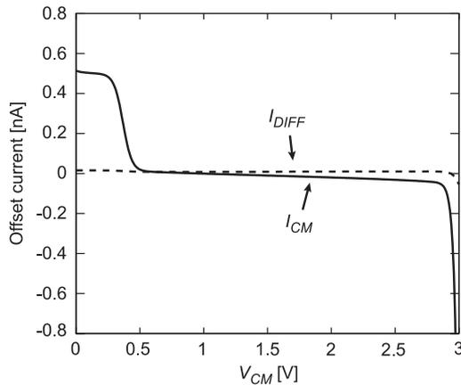
**Fig. 5** Common-mode offset current  $I_{CM}$  and differential offset current  $I_{DIFF}$  as a function of common-mode voltage  $V_{CM}$  for terminals 1 and 2, measured for  $I_b = 1$  nA and  $V_{dd} = 3$  V.
